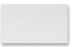
Supercruise styles combine quality high tenacity fiber selection with high beat-up constructions for improved stretch resistance, bias stability and fabric recovery. Efficiently woven in a high tenacity polyester and available in wide width for ease of production. With our standard Polypreg finish it can be used across a wide range of applications.
