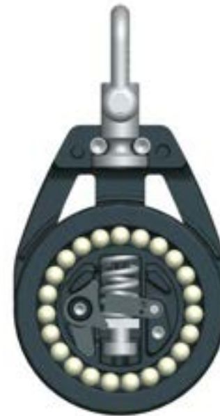
Automatic ratchet block, low load. When the block is low-loaded the ratchet mechanism is disengaged and the sheave spins free.
