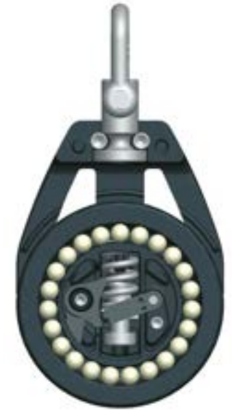
Automatic ratchet block, high load. When the load on the block increases the ratchet engages and the sheave is locked in one direction.
