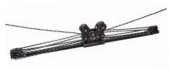
Lead block and cam cleat to be mounted separately in the cockpit, see page 72.
