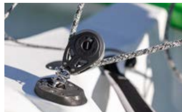
The R60+ features an aluminium sheave that allows for good grip with thin lines.
