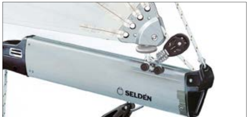
Boom fitted with outhaul car for Seldén furling mast.
