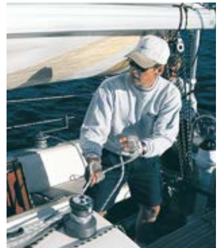
If necessary, apply more main halyard tension.
