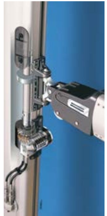
Långedrag 501 equipped with Seldén hydraulic furling mast, hydraulic outhaul and double hydraulic Furlex jib-reefing systems.
