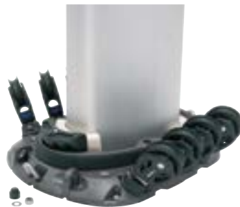
Step the mast and replace the wedge.
